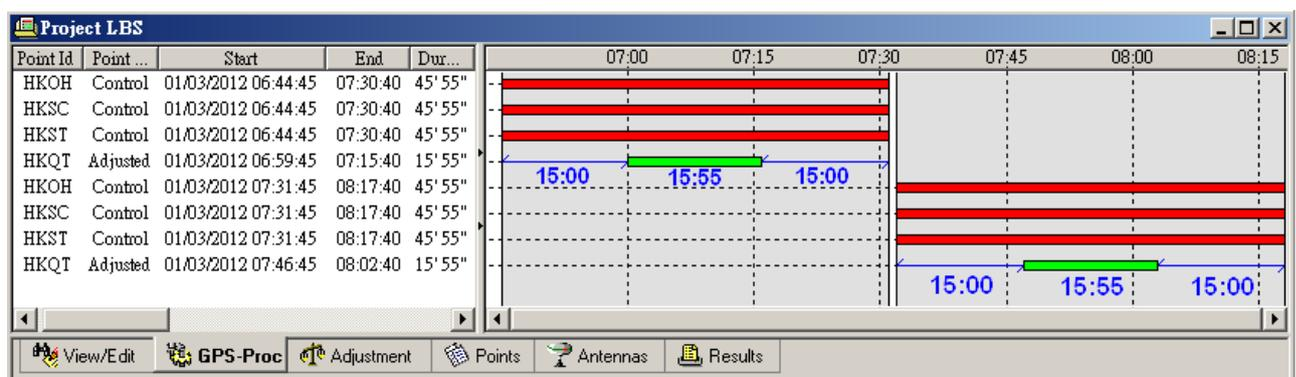
There will be at least 45 minutes observation data at the reference stations, sufficient for LGO to compute an ionospheric model. In case if computed model could not be generated, the Klobuchar model would be used automatically.
